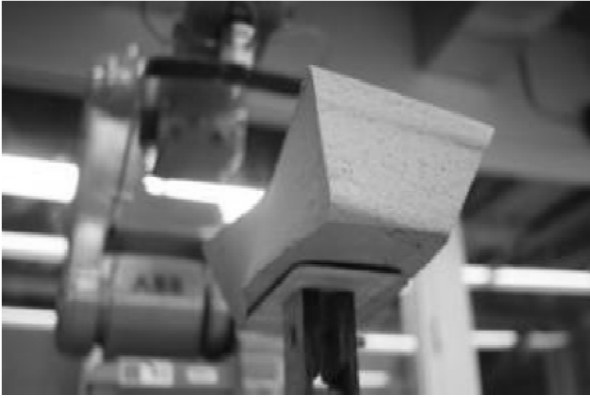
Fig. 11. Wire-cut ruled-geometry ceramic component
