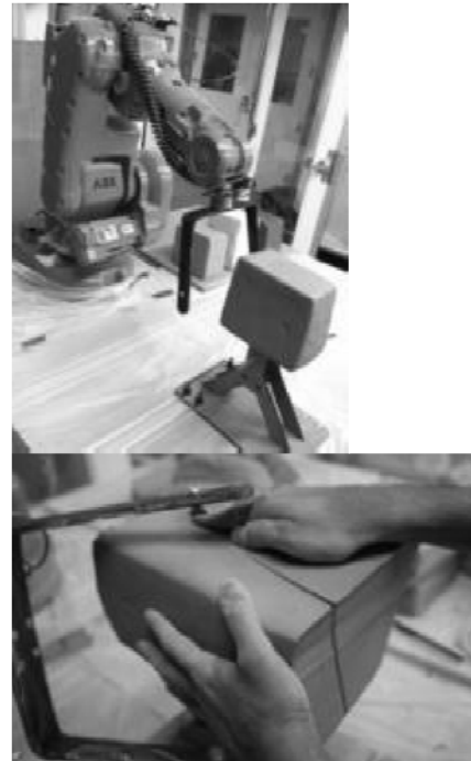
Fig.9. Robotic fabrication of ruled-geometry ceramic components through a wire-cutting tool
