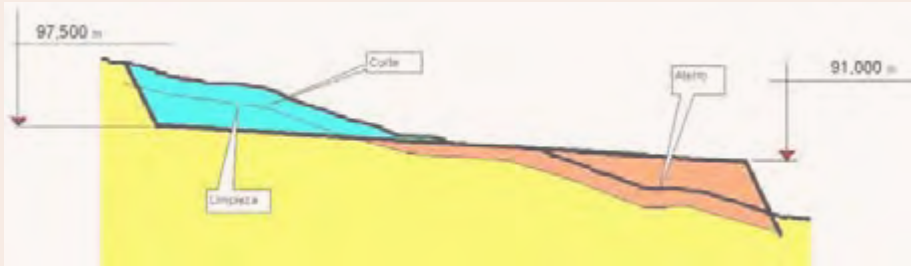
Figure 12: Excavation and filling. / Source: EIA Lot B. Figura 12: Excavación y relleno. / Fuente: EIA Lot B.
