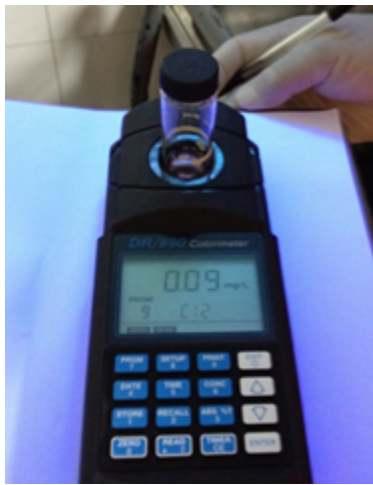
Figure 35: Test to detect residual chlorine Source: picture provided by AERIS
