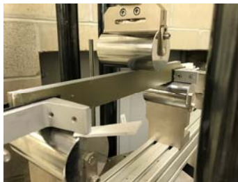
Figure 3: Photograph of material test sample during three-point bending test.
