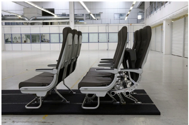
Figure 5: Airbus "Smart Cabin Reconfiguration" system - foldable seats installed along a floor rail
